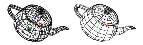
The left image is generated with culling off, while the right image with culling on. Note that there is no hidden surface removal, and that some of the models were not imported with full polygon information, so the culling is occasionally erratic for those.
